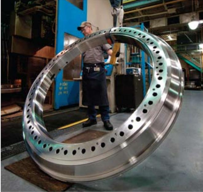
A technician at Timken's Tyger River, South Carolina facility hoists a main-shaft bearing produced at the facility. (Courtesy of The Timken Co.)
